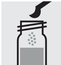
Add 1 level blue micro-spoon of K-2K , close the cell with the screw cap.
