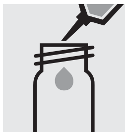
Pipette 5.0 ml of the sample into into a empty round cell (Empty cells, Cat.No. 250621).
