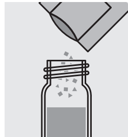
Add the contents of a VARIO Silica HR Acid Rgt F10 powder pack and close the cell with the screw cap.
