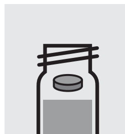
Add 1 tablet Cyanuric Acid , crush with stirring rod, and close with the screw cap.
